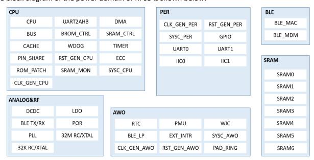
RF03 is composed of 6 power domains which are CPU, PER, BLE, AWO, SRAM and ANALOG.
