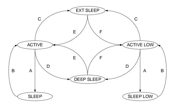
The power state transfer condition in the above diagram is shown in the table below:
