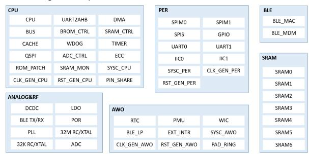
RF01 is composed of 6 power domains which are CPU, PER, BLE, AWO, SRAM and ANALOG.
