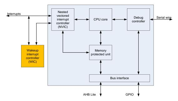
The processor is built on a highly area and power optimized 32-bit processor core, with a 2-stage pipeline von Neumann architecture. The processor delivers exceptional energy efficiency through a small but powerful instruction set and extensively optimized design, providing high-end processing hardware including a single-cycle multiplier.
