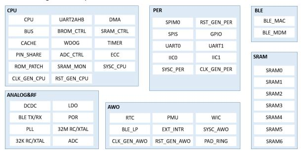
BX2418 is composed of 6 power domains which are CPU, PER, BLE, AWO, SRAM and ANALOG.
