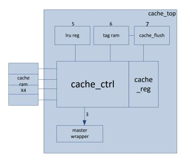
The data RAM size of the cache controller is 16KB and can be shared with the system SRAM if the cache controller is not enabled. The cachable address space is 8MB. The LRU algorithm is implemented in the cache controller to update the cache data. An AHB master wrapper is implemented to convert the cache data access to the SPI command of the QSPI controller.
