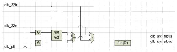
The clock gating on the path of clk\_32m is controlled by the programmable registers 0x20201004[7:6]. The name of the registers are clkg\_hbus\_div\_32m\_clr and clkg\_hbus\_div\_32m\_set. Writing 1 to 0x20201004[7] will close the clock gate(no clock will be output). Writing 1 to 0x20201004[6] will open the clock gate(clock will be output). If the clock divider is not needed by the current system, the clock gate can be closed to save the power.
