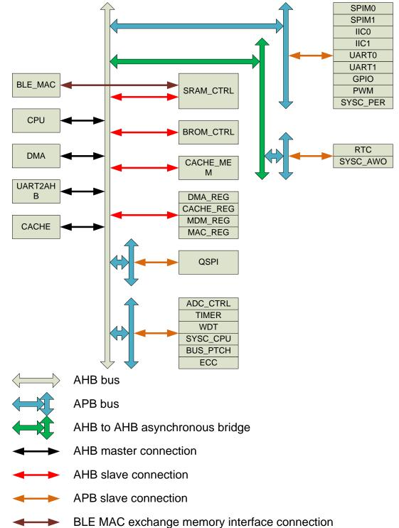
The system bus is based on AHB and APB. The data width of the bus is 32 bits. The AHB bus works under the same frequency with CPU. The maximum frequency of AHB bus is 96MHz
