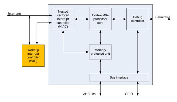
The Cortex-M0+ processor is built on a highly area and power optimized 32-bit processor core, with a 2-stage pipeline von Neumann architecture. The processor delivers exceptional energy efficiency through a small but powerful instruction set and extensively optimized design, providing high-end processing hardware including a single-cycle multiplier.
