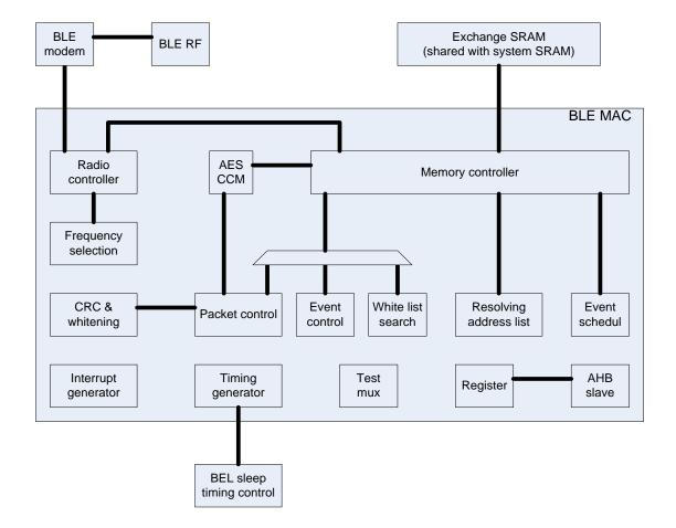
The block diagram of the BLE MAC is shown above. The exchange memory used by the BLE MAC is shared with the system SRAM. This makes the allocation of the exchange memory and the system memory programmable. The maximum addressable size of the exchange memory is 32KB which is addressed at 0x00128000 of the system address space. The exchange memory contains the exchange table, control structures, TX/RX descriptors and the associated data buffers, and RAL structure.
