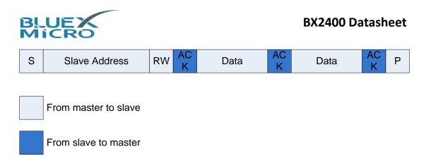
If the master is receiving data then the master responds to the slave-transmitter with an acknowledge pulse after a byte of data has been received, except for the last byte. This is the way the master-receiver notifies the slave-transmitter that this is the last byte. The slave-transmitter relinquishes the SDA line after detecting the No Acknowledge (NACK) so that the master can issue a STOP condition. The following diagram shows the scenario that master is the receiver:
