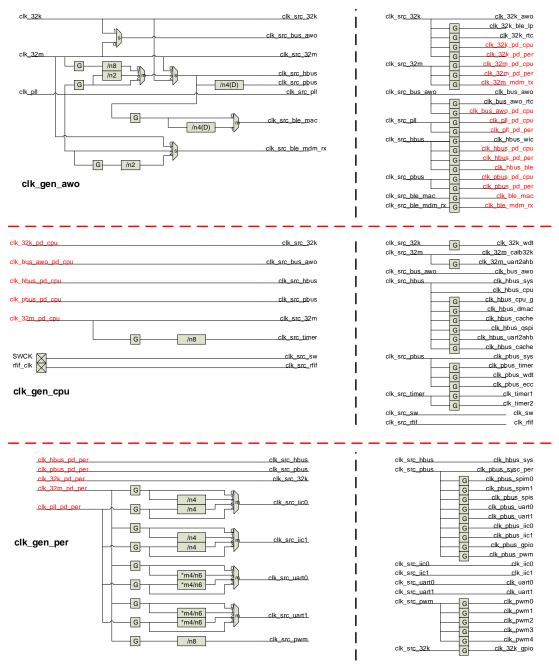
The clock system is comprised of three subsystems which are clk\_gen\_awo, clk\_gen\_cpu and clk\_gen\_per. Clk\_gen\_awo is in the AWO power domain and
