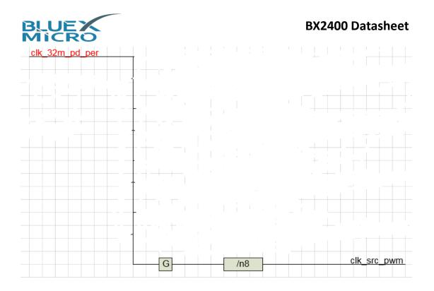
The clock gate is controlled by register 0x20149014[1:0] which is named as clkg\_clr\_pwm\_div and clkg\_set\_pwm\_div. Writing 1 to 0x20149014[1] will close the clock gate(no clock will be output). Writing 1 to 0x20149014[0] will open the clock gate(clock will be output). If the clock divider is not needed by the current system, the clock gate can be closed to save the power.
