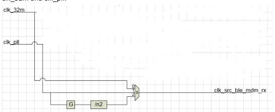
Clk\_src\_ble\_mdm\_rx is the receiving clock for the BLE modem. It comes from clk 32m and clk pll.
