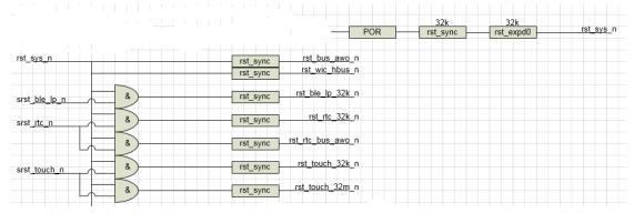
Some of the reset signals can be pull low by software reset and some signals can not be pulled low. The software reset signal is "AND" with the global reset signal and then synchronized to the clock domain of the target module. The reset signals of modules are shown in the table below:
