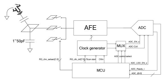
The touch controller controls the analog touch module, captures the touch ADC output and generates the touch interrupt which is used to wake up the system when system is in deep sleep or extended sleep mode. The touch controller is composed of three parts, the clock divider, the time counter and the ADC controller.
