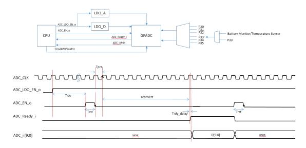
The ADC controller controls the analog module multiple channel ADC, samples the ADC data and pass the data to the CPU through the APB bus interface. The block diagram of the ADC controller is shown below:
