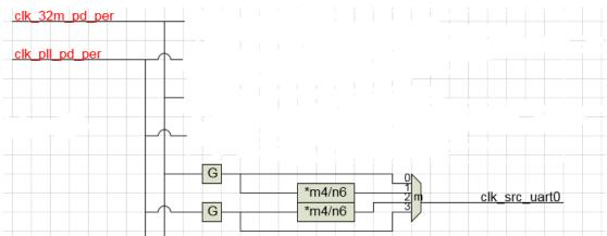
The clock gate on the path of clk\_32m is controlled by register 0x20149010[9:8] which is named as clkg0\_clr\_uart0 and clkg0\_set\_uart0. Writing 1 to 0x20149010[9] will close the clock gate(no clock will be output). Writing 1 to 0x20149010[8] will open the clock gate(clock will be output). If the clock divider is not needed by the current system, the clock gate can be closed to save the power.
