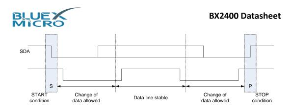
The data line SDA can only changes when the clock line is low except for the START and STOP condition.
