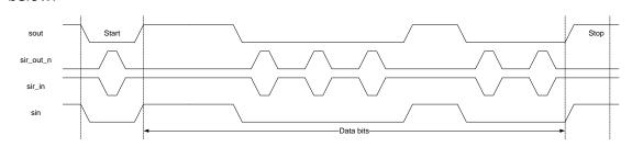
The bit format is not the same as the UART. In IrDA, transmitting a single infrared pulse indicates logic 0, Non-transmission of a pulse indicates logic 1. The width of each pulse is 3/16ths of the serial bit time defined in chapter 34.3. Thus, each frame begins with an infrared pulse for the start bit. However, received data is inverted from transmitted data due to infrared pulses energizing the photo transistor base of the IrDA receiver, which pulls its output low.
