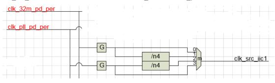
Clk\_src\_iic1 is the clock for IIC1. It is from clk\_32m and clk\_pll.
